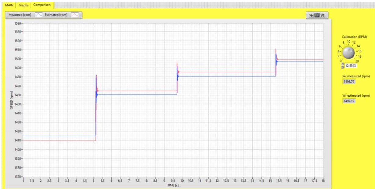
Figure 8. Front panel of the virtual instrument for measurement and estimated speed (load torque is step decreased)
