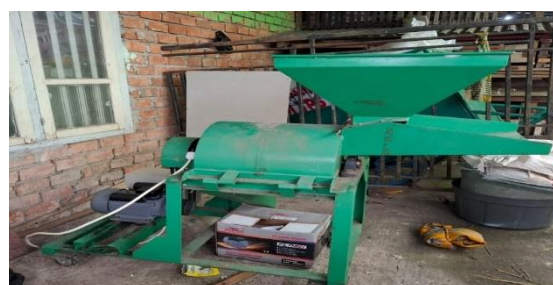
Figure 6. Waste Shredder Machine Modified with an Electric Motor
