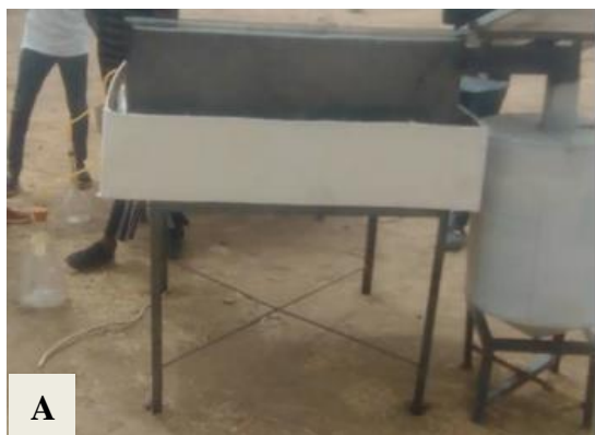
Figure 2. Snapshot of the Solar Stills (a) Modified Passive Still Distiller (b) Modified Convectional Still Distiller
