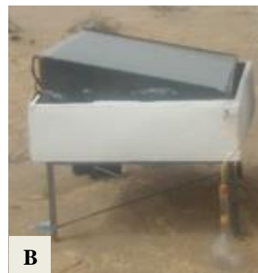
Figure 2. Snapshot of the Solar Stills (a) Modified Passive Still Distiller (b) Modified Convectional Still Distiller
