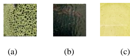
Fig. 3 Comparison of label appearance with a solution : (a) stored 0 hour [10], (b) stored 3 days at room temperature [10], and (c) stored 3 days at 7^{\circ}\text{C} (this experiment)
