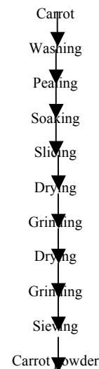
Fig 1: Flow diagram for the production of carrot powder for colouring and flavouring
